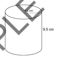
One equation for calculating the volume of a cylinder is V = Bh, where B represents the area of the base of the cylinder. Which expression can be used to find the value of B, in square centimeters, for this cylinder?
